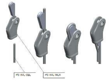
PS-HVL-WE1 Wire Ending installation is done with bolt washer and nut. The installation is completed with  $\emptyset$ 19 mm wrench.
